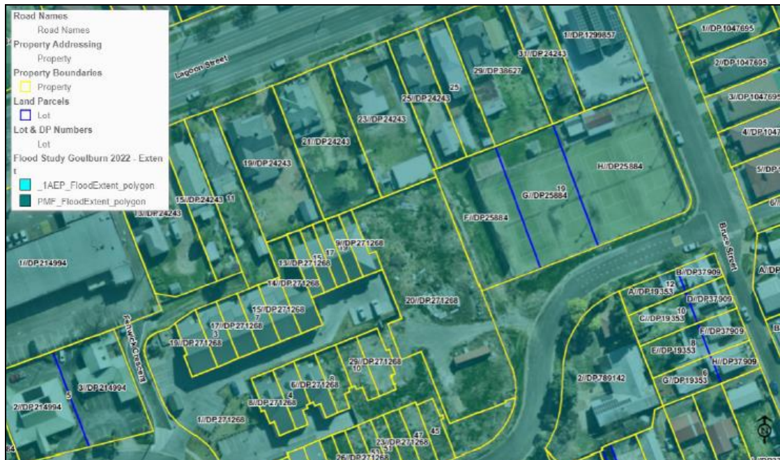
Figure 3-2 – 1% AEP Flood Extent
